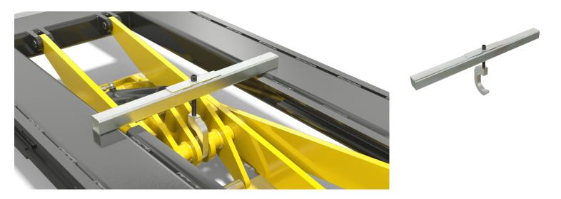
The UnoLiner W50 Manual Lift fixes a scissor lift to its bench frame. In combination with the W10 Bench Wheel Set, this bracket provides mobility for UnoLiner's Drive-On and Roll-Over chassis straightening benches. This makes moving the bench to another spot in the workshop fast and easy. Transporting to another location also becomes an option with this combination, because a secured bench and lift can be loaded onto a truck.
