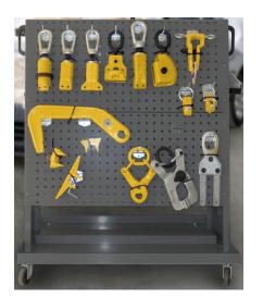
For storing clamps and assorted accessories, the V20 Trolley for Clamps is the perfect fit. Keep your workshop organized with this mobile storage rack, equipped with caster wheels. This way, you can keep your chassis straightening tools ready for use while saving space in the process. Clamps and tools sold separately.
