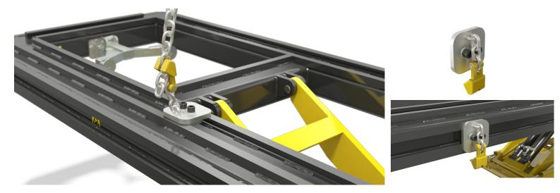
The UnoLiner D15T Chain Guide has been developed for two-way locking straightening benches, such as the CRS4600T and CRS6000T. This handy chain holder slides into both the straightening benches' top and side profiles. Tighten its two bolts to secure it firmly onto the bench and attach a pulling chain to the integrated chain holder tool. Its special design with chain tension guide allows for pulling from many directions.
