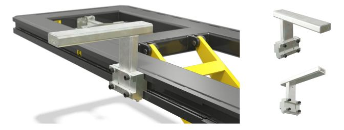
The UnoLiner B70 Adjustable Bench Adapter has an adjustable height of 60 to 330 mm above bench level and fits on all UnoLiner straightening benches. The B70 supports all types of UnoLiner chassis clamps and allows for maximum flexibility when it comes to repairing all sorts of vehicles, from the smallest microcar to the largest SUV, MPV, or heavy-duty pickup truck.
