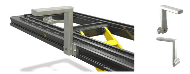
Designed to accommodate the Shark Measuring System, the UnoLiner B10S Shark Bench Adapter has been outfitted with heightened chassis clamp arms. This way, a Shark Measuring beam fits between bench frame and vehicle. Also suitable for other measuring systems or for users who prefer the additional work height. Like the standard B10 Bench Adapter, the B10S comes equipped with the Quick Lock one-bolt locking system.
