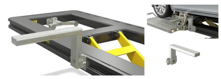
The UnoLiner B1055 Bench Adapter has been specifically developed for vehicles with larger track and chassis widths. The B1055 has the same height as the standard *B10 Bench Adapter* and its chassis clamp arms have been elongated without sacrificing strength. The B1055 is suitable for all UnoLiner chassis clamps and straightening benches. Its patented Quick Lock one-bolt locking system makes attaching the B1055 easy and safe.
